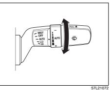
If the control lever has on "AUTO" position, you can increase the system's sensitivity to rain/snow by turning the knob of the control lever forward for increased sensitivity or rearward for decreased sensitivity.
